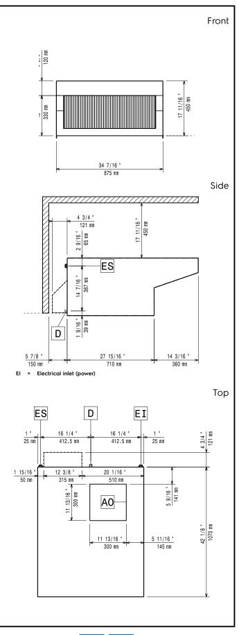
Ventilation Equipment Standard hood (with fan motor) for 6 & 10 GN 1/1 lenghtwise combi ovens
